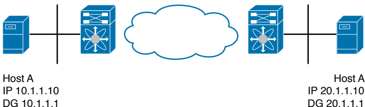
Figure 20-7 Two Hosts in Different Subnets
