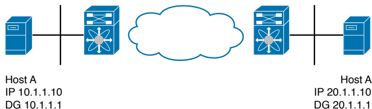
Figure 20-2 Communications Between Two Hosts in Different Subnets
