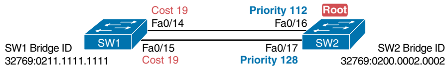
Figure 8-7 The Need for Additional Root Port Tiebreakers
