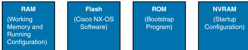
Figure 5-10 Cisco Switch Memory Types
