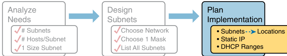
Figure 11-21 Facts Supplied to the Plan Implementation Step
