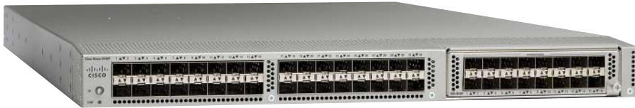
Figure 5-1 Cisco 5500 Nexus Switch Series
